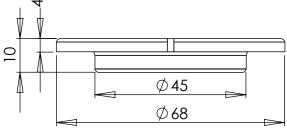
The mounting diagram shows the mounting hole and central hole locations and sizes.
