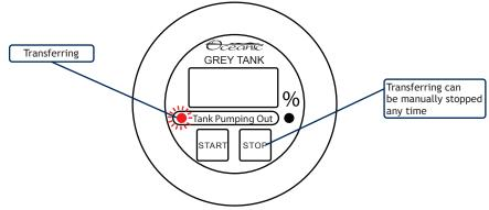
If the ship's power is removed during transfer the transfer will stop. For safety reasons when the power is restored the unit will NOT restart the transfer unless the START button is pressed again or the automatic start feature is enabled and the tank level is below the user settable threshold.
