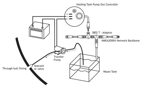
The power control cables on the back of the 3350 HTPO should be connected to the "C" and "NO" terminals.
