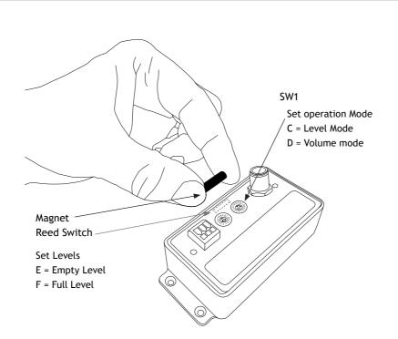
The 4-20mA Tank Level Adaptor can be calibrated to operate between the set **Empty & Full level.**
